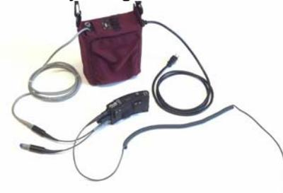
Disconnect the gray plug from the Y Cable or FlowMaker Controller and plug it into the gray receptacle on the Reserve Battery/Charger.
