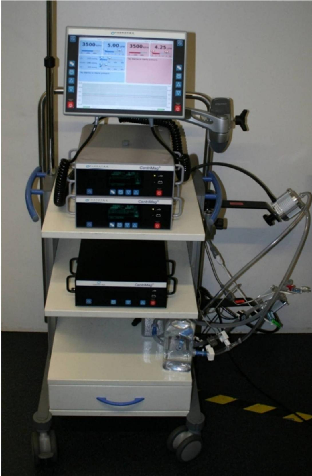
**Figure 14: System Cart, Primary & CentriMag Back-Up Consoles and Mag Monitor. Also shown are two water filled training loops connected to CentriMag pumps.**
