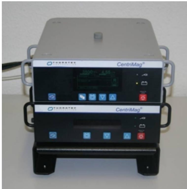
**Figure 46: Primary & CentriMag Back-Up Consoles Mounted on Portable Stand Illustrating the Univentricular Support Configuration**
