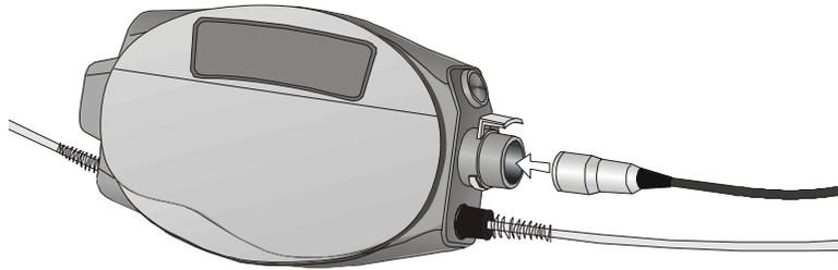
**Figure 5.10: System Controller to LVAD Percutaneous Cable**
