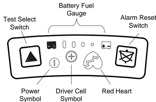
**Figure 4: HeartMate II System Controller User Interface Panel**
