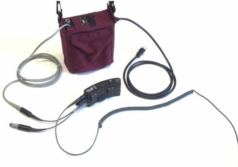
Figure 21 Reserve Battery/Charger Connected to Y Cable then FlowMaker® Controller
