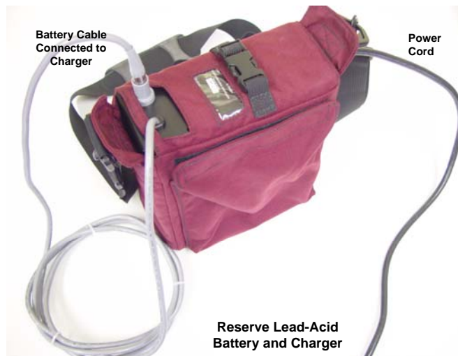
Figure 22 Charging the Reserve Battery/Charger
